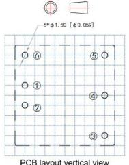
PCB layout vertical view Grid 2.54x2.54[0.10x0.10]
