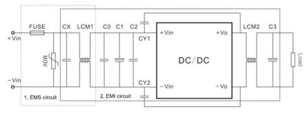
Note: Part 1 in the circuit diagram is for EMS, part 2 for EMI filtering, both can be adjusted according to the actual situation.
